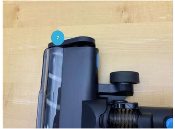
Push up the end cover (pos. 2) for rotating brush.
